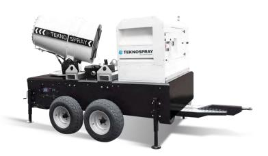
TeknoSpray, part of the Trime Group, has developed a wide range of innovative, versatile and compact dust suppression systems. Fully automatic with R.O.T. system standard - Remote control, automatic Oscillation 0-340° and electric Tilting system. Used in mines, quarries, demolition, recycling and odor removal.
